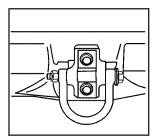
Your vehicle has two recovery loops at the front of the vehicle and one at the rear of the vehicle. You may need to use them if you are stuck off-road and need to be pulled to some place where you can continue driving.
